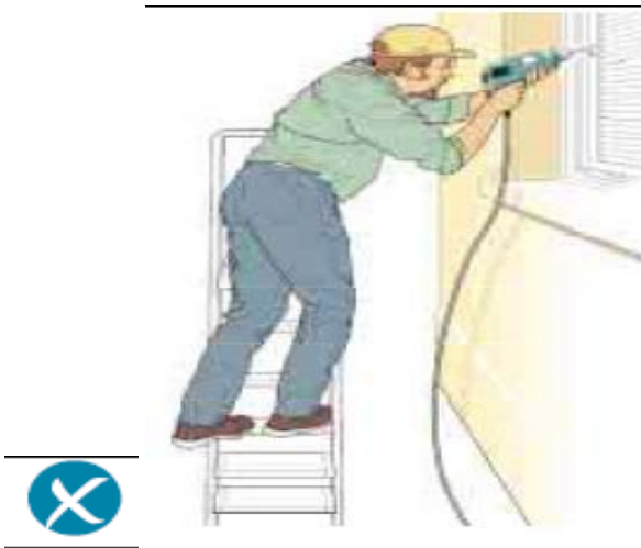
Incorrect – steps side on to work activity
